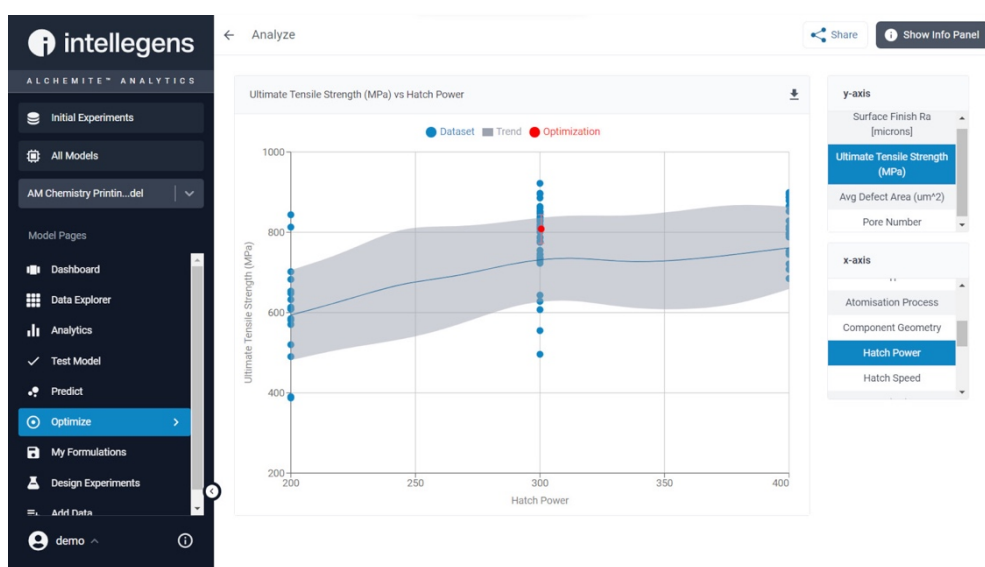
Figure 3. Alchemite™ Analytics web user interface: analysis of additive manufacturing data.
